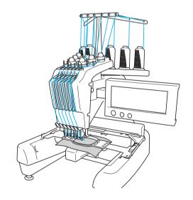
Not all six needles can be used to sew at the same time. Only one needle is moved to the embroidering position at a time. According to the sewing order, the needle bar case is moved to the left and right so that the needle bar and needle thread with the required color can be moved to the embroidering position.
